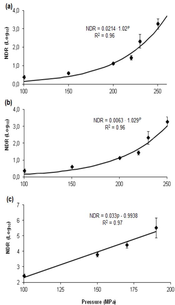
Figure 2. Inactivation kinetics of *Lactobacillus helveticus* (a), *Listeria innocua* (b) and *Pseudomonas fluorecens* (c) inoculated in skimmed milk and processed by high pressure homogenization (n = 3)
