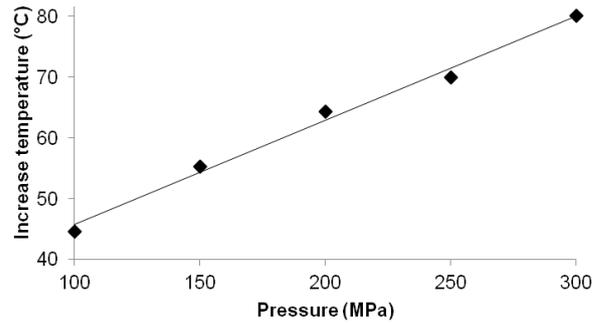
Figure 1. Temperature increases in skimmed milk samples processed by high pressure homogenization .Inlet temperature = 23.0 ± 1.0°C. Results shown are mean of triplicate trials on individual milk samples
